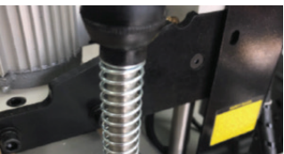
Step and Repeat Operation Index Pins (Left and Right)
